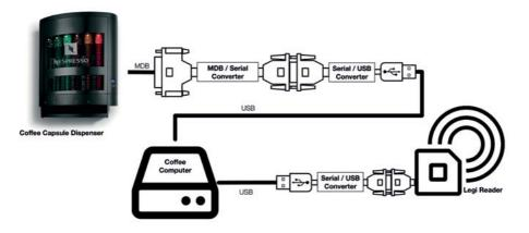
Figure 2: Post-incident hardware setup
